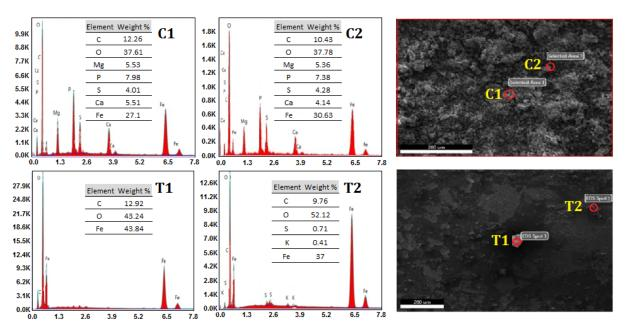
Figure 3. EDS analysis spectrum and the chemical composition for the deposits formed on N80 steel samples incubated in SRB contaminated anaerobic environment for 90 days at 37 °C (Control) (C1 and C2), and incubated in SRB contaminated anaerobic environment for 60 days at 37 °C then treated by biocide2 CHIMEC 7660 and left for another 30 days at 37 °C (Treatment) (T1 and T2).
